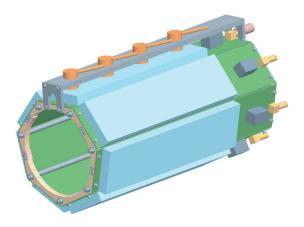
**FIGURE 3.** Mounting geometry for the scintillators surrounding the mixing region. For the measurements reported here, three of the seven modules were replaced with two layers of position sensitive silicon strip detector. The small detectors (orange) are CsI crystals for looking at positron annihilations. A similar, seven-segment scintillation detector surrounds the degrader foil.
