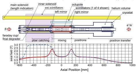
**FIGURE 1.** Schematic diagram of the ALPHA apparatus. The graph shows the on-axis longitudinal magnetic field due to the solenoids and mirror coils. The blue (red) curve is the field with (without) the inner solenoid energized.
