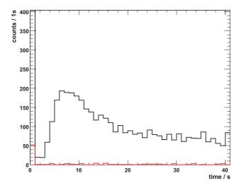
**FIGURE 4.** Scintillation triggers versus time after the start of mixing for normal mixing (black) and for the same sequence but without positrons present (red). The octupole was at 900 A, corresponding to a trap depth of about 0.5 K, for these measurements.
