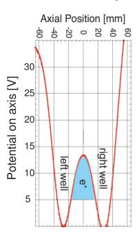
**FIGURE 5.** Potential on the axis of the nested well used for positron-antiproton mixing. The antiprotons are injected into the nested well with a potential of about 23 V on this diagram. The blue shaded region represents the approximate spacecharge potential of the positron cloud.
