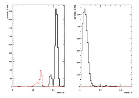
**FIGURE 6.** Antiproton annihilation signals observed while ramping down the left potential wall (left panel) followed by the right potential wall (right panel), after the mixing cycle was completed. The black (red) curves are with (without) positrons. The voltage ramp-down rate is about 70 V/s. This signal is for a single mixing cycle with eight AD shots.
