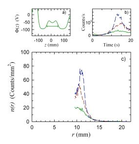
**FIGURE 10.** Comparison of the  $\overline{p}$  radial profile with different density positron plasmas. The green, solid curve shows the profile with no e<sup>+</sup>, and the red short-dash and blue long-dash curves show the profile with 13 million and 25 million e<sup>+</sup> respectively. The well length was  $85 \pm 5$  mm, the maximum field was 1.20 T, and the ramp time was 20 s. The graph descriptions and all other parameters are the same as in Fig. 9.
