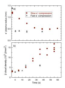
**FIGURE 4.** The a)  $e^-$  radius and b)  $\overline{p}$  density as a function of time, for fast and slow compression. Note that the  $\overline{p}$  density does not track the  $e^-$  compression if the latter is fast.
