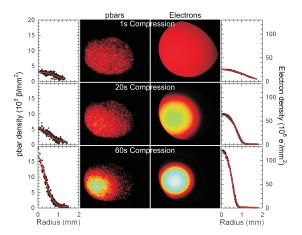
**FIGURE 2.**  $\overline{p}$  and  $e^-$  images showing the effects of compression, and the resulting radial profiles. The red lines are Gaussian-like (i.e.  $\exp(-|r/r_0|^k)$ ), where  $k \approx 2$ ) fits to the radial profiles. The sharp boundaries are caused by apertures.
