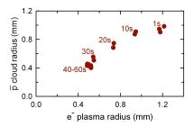
**FIGURE 5.** The  $\overline{p}$  cloud radius as a function of the e<sup>-</sup> plasma radius for the slow compression data shown in Fig. 4.
