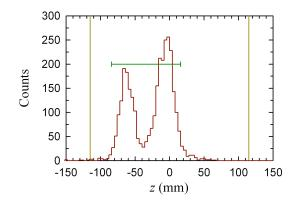
**FIGURE 8.** Axial positions where the  $\overline{p}$ 's hit the trap wall under the influence of the octupole. The horizontal bar indicates the the axial extent and position of the electrostatic well confining the  $\overline{p}$ 's. The loss is greatest near the ends of the confining electrostatic well. The positions are determined by a position-sensitive particle detector which monitors the  $\overline{p}$  annihilation products; the vertical bars indicate the axial extent of the detector.
