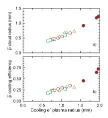
**FIGURE 3.** a) The cooled  $\overline{p}$  cloud radius as a function of the radius of the e<sup>-</sup> plasma. The various symbols correspond to trials with differing total electron numbers (100-165 M). b) The cooling efficiency (see text) as a function of the e<sup>-</sup> plasma radius.
