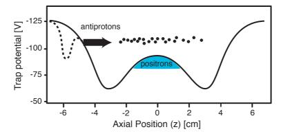
**FIGURE 1.** Nested trap configuration of the mixing trap for mixing positrons and antiprotons for antihydrogen formation. The potential on axis is given. The dashed curve indicates the potential before injection of the antiprotons.
