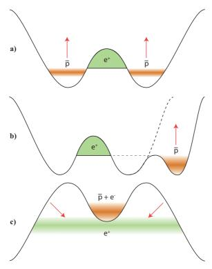
**FIGURE 9.** Examples of suggested mixing schemes for creating antihydrogen cold enough to trap. a) The antiprotons that accumulate in the sidewells may be slowly reinjected to interact with the positrons at low relative energies. b) The initial injection of antiprotons may be attempted at low relative energy, possibly directly from the sidewell with electrons to keep the antiprotons cold. c) The antiprotons are kept cold while the positrons are injected.
