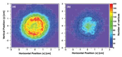
**FIGURE 3.** Cross sectional distribution (xy) of all antiproton annihilation vertices registered during cold (a) and hot (b) mixing. The black dashed circles mark the position of the trap walls. The cylindrical traps have a diameter of 25 mm.
