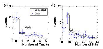
**Fig. 5.** Comparisons of the events measured in the trapping experiment with the distributions of (a) number of tracks per event and (b) number of hits per event, produced by combining the calibration samples with the expected weights (see text). The uncertainties in the distributions are based on the uncertainties in the weighting factors, and the error bars on the data are the counting errors.
