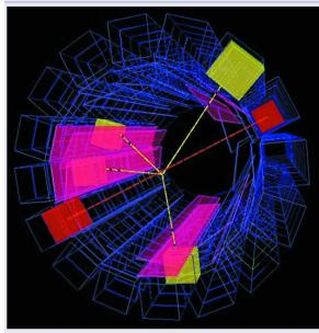
This event display from the ATHENA experiment at CERN shows an antihydrogen atom that has annihilated after striking the wall of the Penning trap (centre, not shown). The nucleus of the anti-atom – the antiproton – annihilates into four charged pions (yellow tracks) that are detected with silicon microstrips (pink), while the positron annihilates into two back-to-back photons (red tracks) that are detected by caesium-iodide crystals (red cubes).
