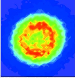
In 2002 ATHENA researchers produced the first cold atoms of antihydrogen, opening the possibility of comparing antihydrogen atoms with ordinary hydrogen. This image shows the transverse density of antiproton annihilation events integrated along the *z*-direction of a cylindrical Penning trap: red indicates high antiproton density; blue indicates low. The red ring corresponds to the inner wall of the Penning trap, which has a radius of 1.25 cm.
