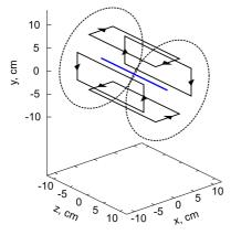
Figure 3. Set of coils used in our numerical simulations: quadrupole coils (solid) with current directions shown with arrows and mirror coils (dashed). The solenoid creating a constant background field is not shown.
