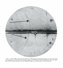
**Figure 1.2:** Left: Carl David Anderson (September 3rd 1905 - January 11th 1991). Right: Photograph of the first observation of a positron. The image was acquired during a cloud chamber study of cosmic rays. The particle track (indicated by arrows and coming from below) was interpreted as a 63 MeV positron passing through a 6 mm lead plate and emerging as a 23 MeV positron (Anderson, 1933).
