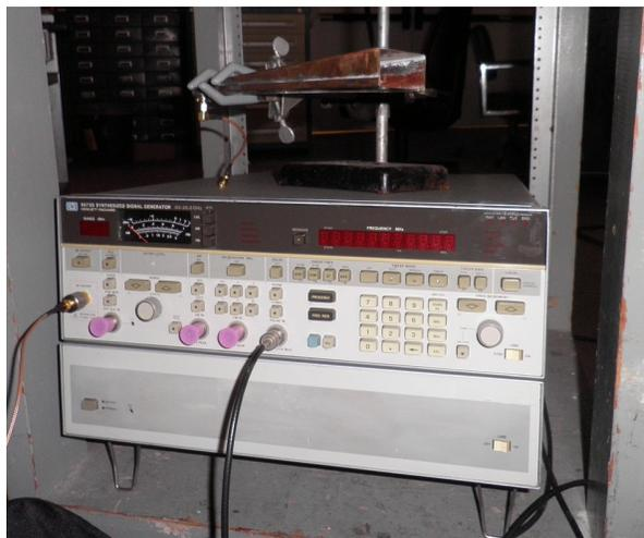
Figure 2.9: Microwave horn sitting on the hp8673d synthesizer used for most of the microwave work in this thesis. Horn was designed and built by the undergraduate Ryan Mcpeters.
