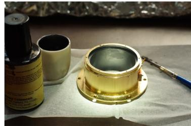
Figure 2.3: An electrode painted with colloidal graphite. Using a paint brush instead of aerosolizing the graphite can produce splotchiness, but these features are only a few microns deep, so they seem to be harmless.
