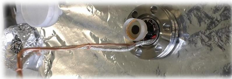
*Figure 4.33: A photograph of the assembled mirror flange. The flange adapter contains holes to allow the space in the bellows behind it to be pumped, but it is an acknowledged pumping restriction. The mirror, piezo, and adapter are bonded using EPOTEK T7109 epoxy.*
