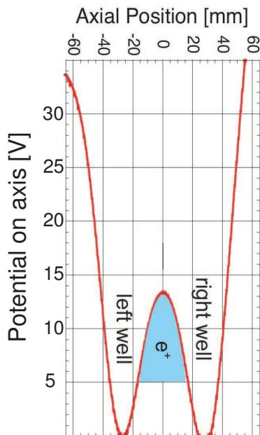
**FIGURE 5.** Potential on the axis of the nested well used for positron-antiproton mixing. The antiprotons are injected into the nested well with a potential of about 23 V on this diagram. The blue shaded region represents the approximate spacecharge potential of the positron cloud.
