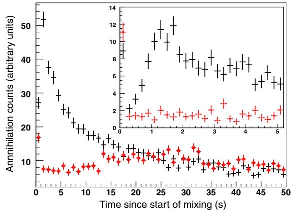
**Figure 4.** Scintillation events as a function of time after the start of mixing, for normal mixing (black) and mixing with heated positrons (red). The time bins are 1 s long. The data are for 10 mixing cycles, normalized to one cycle. The inset is a plot of the first 5 s of the same data, re-binned into 200 ms bins to illustrate the rise time of the antihydrogen production. The uncertainties reflect counting statistics only (1 standard deviation).
