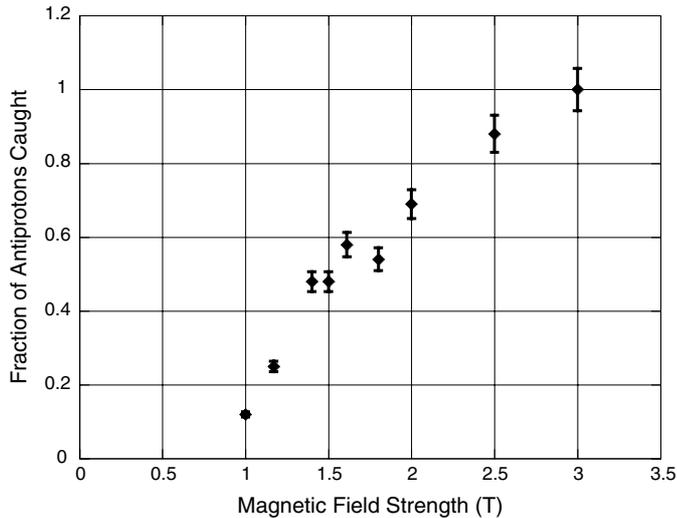
**Figure 2.** Relative antiproton capture efficiency versus magnetic field strength. The measurements are relative to the result for 3 T. The uncertainties reflect counting statistics only (1 standard deviation).
