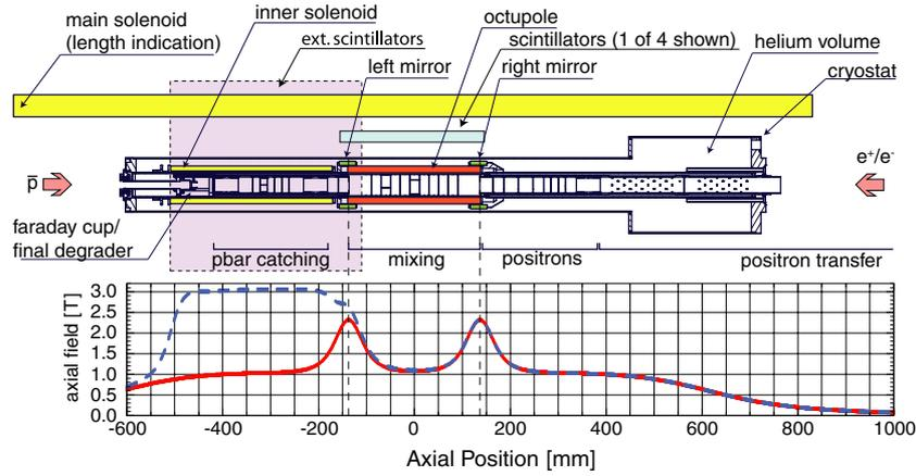
**Figure 1.** Schematic diagram of the ALPHA apparatus. The graph shows the on-axis longitudinal magnetic field due to the solenoids and mirror coils. The blue (red) curve is the field with (without) the inner solenoid energized.
