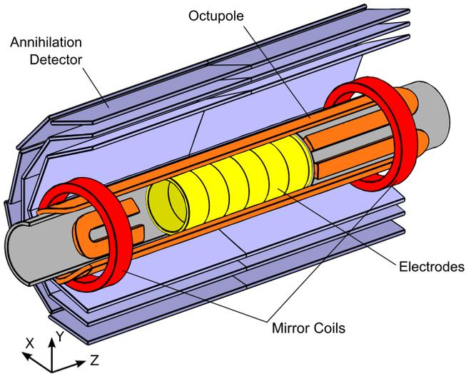
**Fig. 1.** A schematic, cut-away diagram of the antihydrogen production and trapping region of the ALPHA apparatus, showing the relative positions of the Penning-Malmberg electrodes, the minimum-B trap magnets and the annihilation detector. The components are not drawn to scale.
