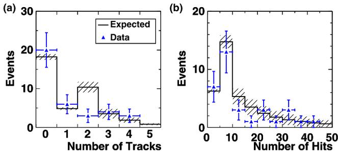
**Fig. 5.** Comparisons of the events measured in the trapping experiment with the distributions of (a) number of tracks per event and (b) number of hits per event, produced by combining the calibration samples with the expected weights (see text). The uncertainties in the distributions are based on the uncertainties in the weighting factors, and the error bars on the data are the counting errors.
