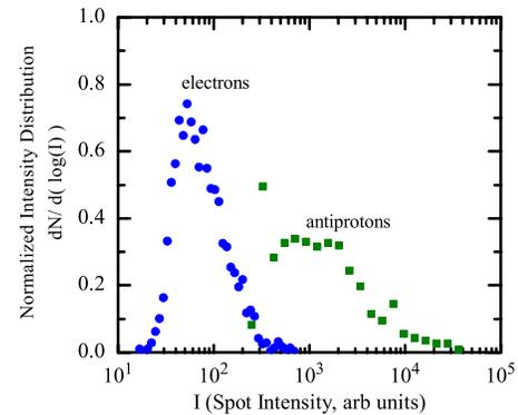
FIG. 3. (Color online) Normalized  $[\lim_{I \rightarrow \infty} N(\log I) = 1]$  electron and antiproton spot intensity distributions. For both species, the MCP front-to-back voltage was 900 V; the impact energy was 200 eV. These parameters maximize the gain.
