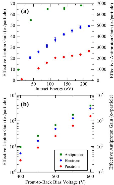
FIG. 5. (Color online) Effective gain of the MCP for different species of particles while varying the voltages on the front and back plates. Particles are extracted from the trap at  $\sim 100$  eV and accelerated by the front plate voltage. In (a), the front-to-back voltage bias was kept constant at 500 V, while impact energy is varied; in (b), the front-to-back voltage bias is varied while the impact energy is held at 200 eV. The uncertainties in the measurements in (b) are  $<2\%$ .
