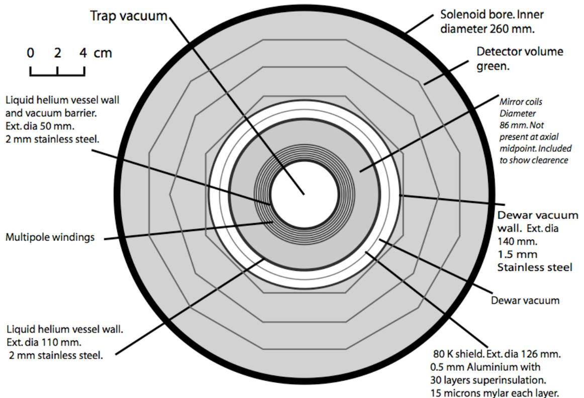
**FIGURE 4.** Cross-section of the apparatus in the mixing region.
